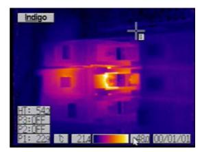
Infrared scan showing abnormal heat being generated in a molded case breaker.
